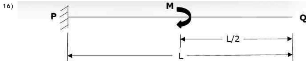
A cantilever beam PQ of uniform flexural rigidity ( $EI$ ) is subjected to a concentrated moment  $M$  as shown in the figure. The deflection at the free end Q is:
